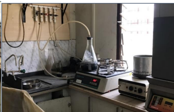
Picture 8: Removal of air voids from loosened asphalt sample
