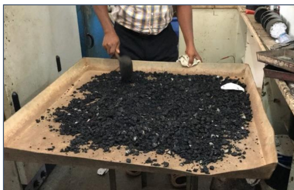
Picture 7: Size reduction of the asphalt core samples
