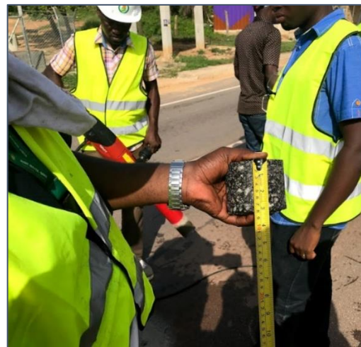
Picture 4: Measuring Extracted Asphalt Core Sample
